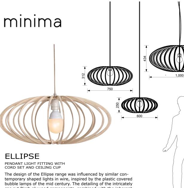
cnc cut Birch plywood components, combined with the inherent elasticity and tension in the timber, allows the light fitting to be easily clipped together without the need for glue or fastenings.
